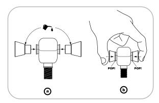
6. Use a small squirt of WD-40 on spacers and insert into boot and heim-joint end. Spacers will subtly pop into place.
