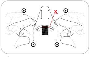
4. The neck of the boot must be pulled down past [x] in figure above. Remove fingers carefully.
