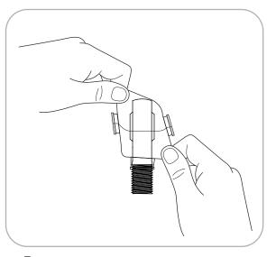
5. Center heim-joint inside of boot for proper fit and hole alignment.
