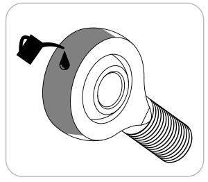
1. Lubricate outside of heim-joint with all purpose grease as shown.
