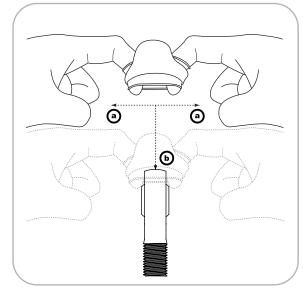
3. Stretch open neck of boot and pull down over lubricated heim-joint.
