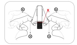
4. The neck of the boot must be pulled down past [x] in figure above. Remove fingers carefully.
