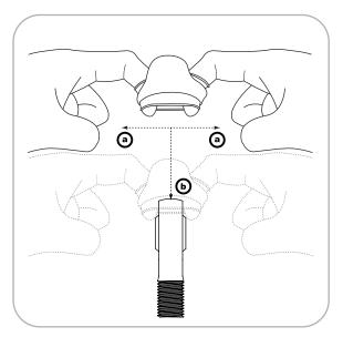
**3.** Stretch open neck of boot and pull down over lubricated heim-joint.
