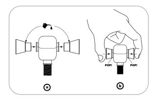
6. Use a small squirt of WD-40 on spacers and insert into boot and heim-joint end. Spacers will subtly pop into place.
