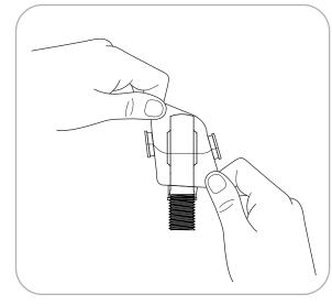
5. Center heim-joint inside of boot for proper fit and hole alignment.
