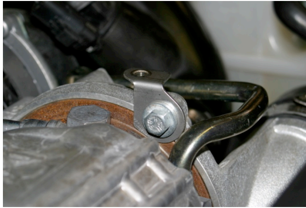
3. Torque bolt to 20Nm (15ft-lbs.). Top surface should be horizontal. Correct as necessary.
