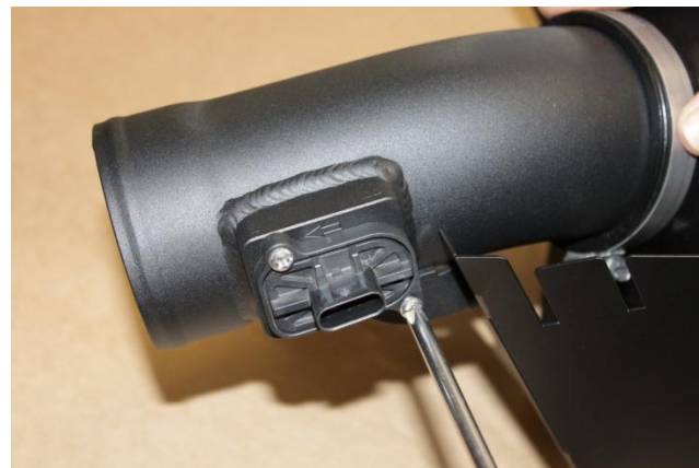
9. Install MAF sensor to NM Intake Pipe using supplied Philips head M4x14mm screws.
