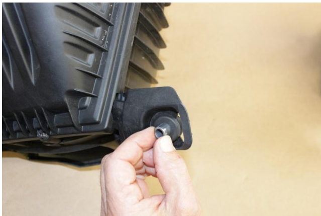
6. Mount NM Intake Pipe to Heat Shield using SS M6x12mm bolts and M6 lock nuts supplied. Now attach and tighten NM Air Filter.
