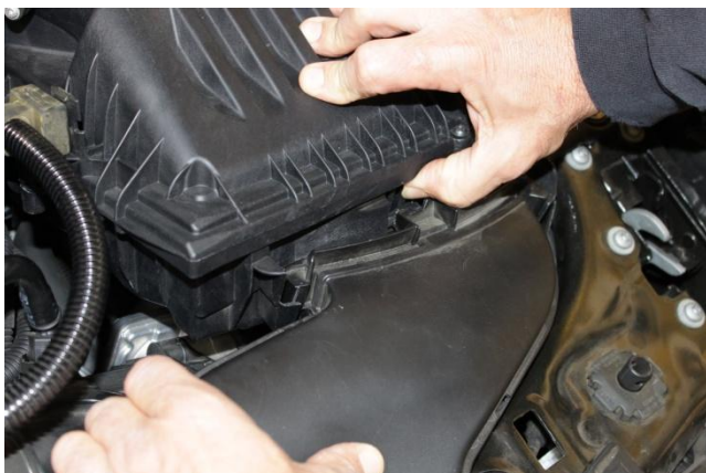
2. Disconnect rubber support for battery cable from air filter box.
