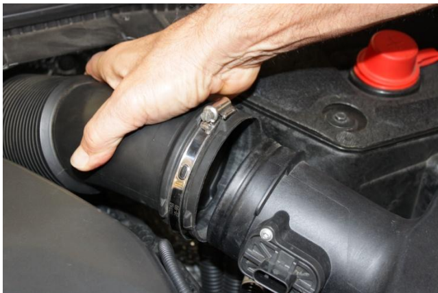
4. Loosen clamp at turbo inlet hose using 7mm Nut Driver and disconnect.
