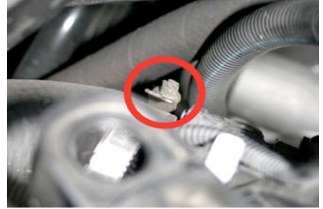
11. Loosen hose clamp and disconnect lower air charge hose from throttle body.
