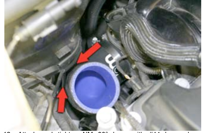
12. Attach and tighten NM 90° hose with #44 hose clamp supplied. NOTE: Keep ample clearance from firewall and brake line.
