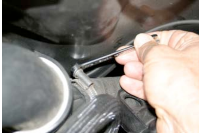
7. Undo hose clamp and remove sound amplifier hose from air charge pipe using a 7mm wrench.
