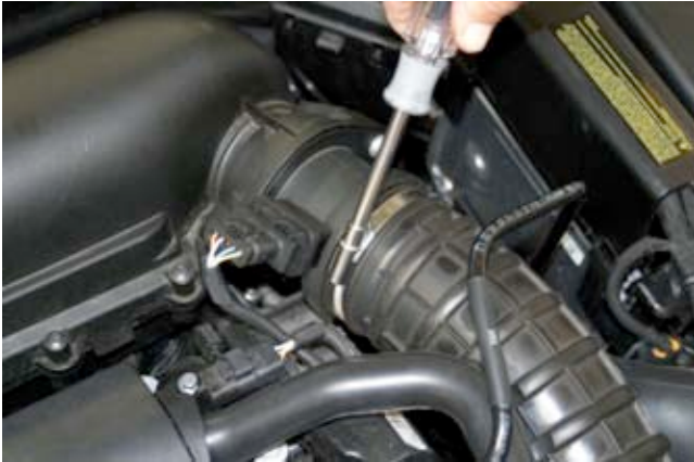
1. Remove OE turbo inlet hose from MAF (mass air flow) sensor. Use screwdriver or 7mm Nut Driver to loosen clamp.
