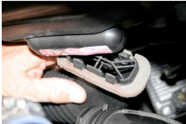
8. Disconnect sound amplifier ducting from firewall by squeezing and pulling down.
