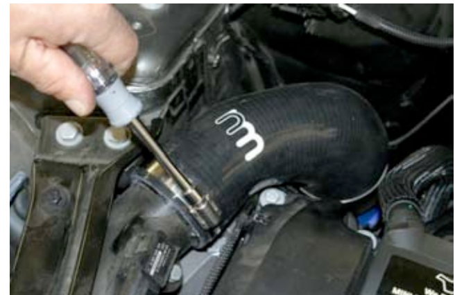
14. Install upper silicone air charge hose with #40 hose clamp and a #44 hose clamp at aluminum pipe and tighten both ends.
