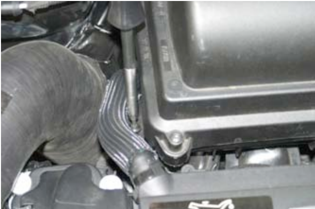
3. Remove T25 TORX screw located on passenger side of air filter box and lift off. NOTE: There are [3] pin mounts that are pushed into rubber grommet mounts on intake manifold, so effort may be required to lift air filter box off of mounts.
