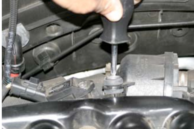
6. Located on back side of intake manifold, remove the Philips screw that retains the sound amplifier.
