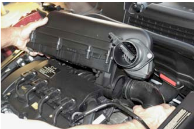
4. Locate fresh air pipe that is attached to air filter box. Disconnect fresh air pipe by rotating the 90° connection counter clockwise and pulling pipe away from air filter box. Remove air filter box from vehicle.
