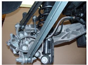
Install NM brake line at caliper and tighten with 11mm line wrench. Push rubber grommet onto rear shock bracket. Install female brake line fitting into bracket at chassis subframe and tighten fitting with an 11mm line wrench.
